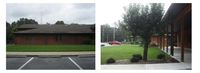
Parking spots south of the church can be replaced with porous asphalt to capture and infiltrate stormwater. Installing rain gardens adjacent to the building can capture, treat, and infiltrate roof runoff. A preliminary soil assessment suggests that the soils have suitable drainage characteristics for green infrastructure.
