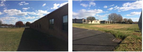
Installing a rain garden adjacent to the north corner of the school can capture, treat, and infiltrate roof runoff. Another rain garden can be installed in the turfgrass area southwest of the school and can treat runoff generated by the parking lot. A preliminary soil assessment suggests that the soils have suitable drainage characteristics for green infrastructure.
